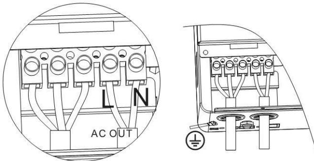
**Note:** The grounding wire shall be as thick as possible (cross-sectional area is not less than 4mm<sup>2</sup>). The grounding point shall be as close as possible to the hybrid solar charge inverter. The shorter the grounding wire, the better.
